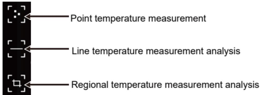
(1) Point temperature measurement: click the point temperature measurement button, and the screen will display the temperature information of three points, namely the central temperature point, the highest temperature point and the lowest temperature point. Click the screen at this time, and the temperature information of the user-defined point will be added.
