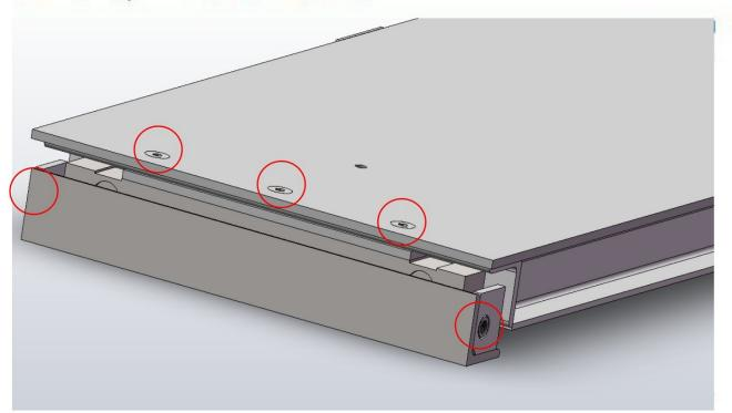
Open junction box and remove load cell wiring. Pull wires through cable holes, and it is suggested to attach fishing wire while pulling out old cell cable. Will help install new load cell cable.
