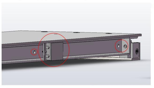
Support frame and remove load cell assembly. Remove two ¾-10 socket head flat bolts from the base plate.
