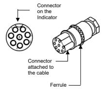
**NOTE:** When moving the scale, take care to prevent bending of the cable and connector too much as over a period of time this can weaken the wires in the connector and cause malfunction.
