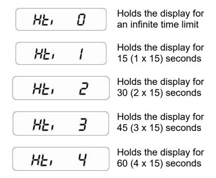
• Press the **[Unit]** key to confirm the selection and move back to the first parameter or press **[Print/Hold]** to exit the parameter setting.
