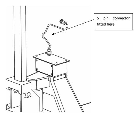
The Indicator bracket is fitted to the PTS using 4 x M4 screws as the picture below shows, these should be tightened using the Allen Key supplied .
