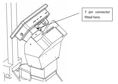
The AE 402 indicator is placed into the mounting bracket, and secured using the two plastic fasteners as shown below:
