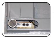
The stainless steel load cells, wiring, and stainless steel junction box are fully protected within the main channel steel via exact cuts made in the channel providing superior protection.
