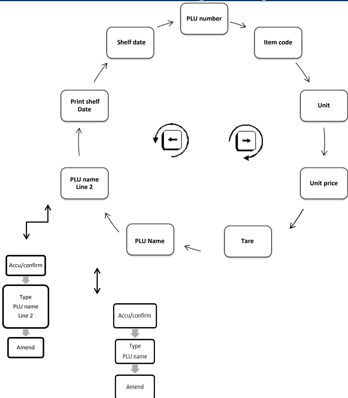
To program a PLU with the F-program press the F-prog and PLU button You can press the right and left arrow keys to navigate up and down the PLU program menu, but you must provide a PLU number. Every PLU has 37 data fields. Many of the fields have been hidden by default. See “Select active PLU fields” for more details.
