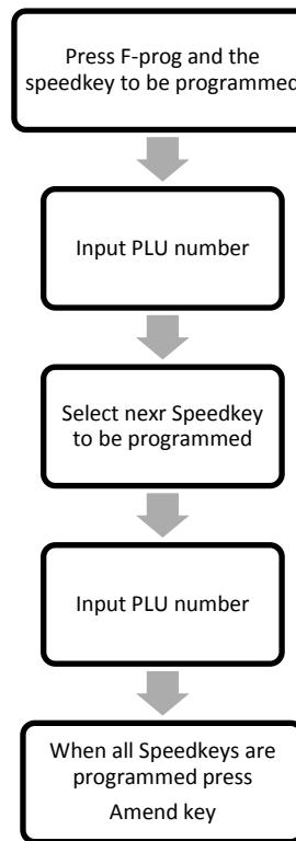
**NB:** To access the second level, press the shift key prior to selecting the speed key
