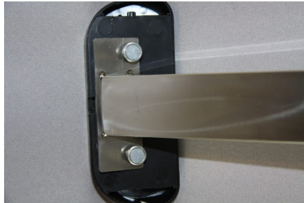
Figure 2.7 Remote Display Attached to Column
