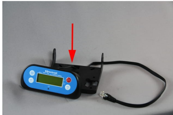
Figure 2.14 Display Cable Routing
