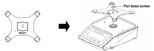
**2** Tighten the "Pan base screw" firmly.
