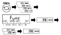
Push [Menu] key, then push [F1-F4] keys to go to <645 SPAN OUT>.
