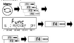
2 Exit the setting menu and operate with "zero-point adjustment reminder".
