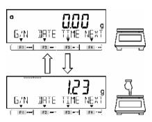
Press the weighing pan lightly to check if the indication changes.
