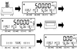
Place the animal on the weighing pan. After the weight variations fit within the set range, the weighing indication is held and < HL 1 > indication appears. Remove the animal, then automatically
