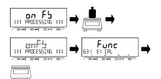
Place the weight in the center of the weighing pan.
