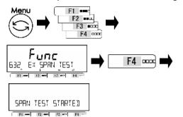
Push [Menu] key, then push [F1-F4] keys to go to <632 EX SPAN TEST>. Push [F4] key to execute.
