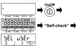
Enable the <642 PASSWORD> and register the administrator password in <643 SET ADMIN PASS>, then power-off the balance. Push [On/Off] key, then the balance shifts to User login mode after start-up operation.
