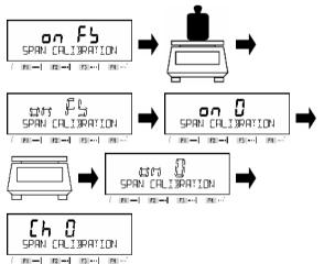
Place the weight in the center of the weighing pan.
