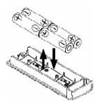
Make sure insert batteries with the positive and negative poles correctly inserted.
