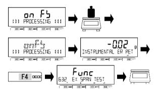
Place the weight in the center of the weighing pan.
