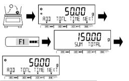
Remove the previous sample to be weighed to return the indication to zero and then place a next sample to be weighed.
