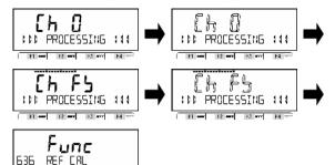
Display changes to the order of "blinking of <Ch 0>"  $\rightarrow$  <Ch FS>  $\rightarrow$
