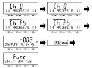
Display changes to the order of <Ch 0>  $\rightarrow$  "blinking of <Ch 0>"  $\rightarrow$  <Ch FS>  $\rightarrow$  "blinking of <Ch FS>"  $\rightarrow$  <INSTRUMENTAL ER> and the instrumental error of the balance is displayed.
