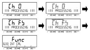
Display changes to the order of <Ch 0>  $\rightarrow$  "blinking of <Ch 0>"  $\rightarrow$  <Ch FS>  $\rightarrow$  "blinking of <Ch FS>"  $\rightarrow$  <633 INT CAL>.
