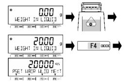
Put the sample on the net/basket in the water/liquid, then push [F4] key to record.
