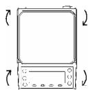
At the time of shipment, the adjusters provided at the four corners of the bottom are locked. Turn them in the direction shown in the figure on the left to loosen them.
