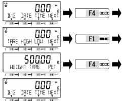
The tare weight can be checked by operating "Free keys" if the <TARE> is assigned to the Free key.
