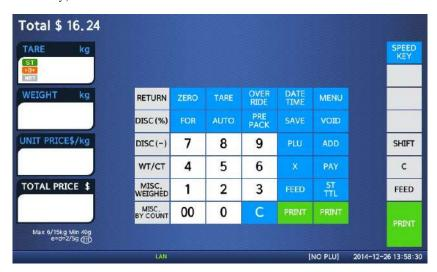
Note: - You can press the VOID key to undo the transaction. (See chapter 3.10).
