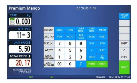
④ Press the PRINT key. Markdown(STRIKE THROUGH)s printed on label as figure.
