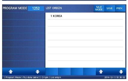
• Press Print Key to List Origins on screen. After Origins are listed on the screen, pressing the TEST key will print the Origins.
