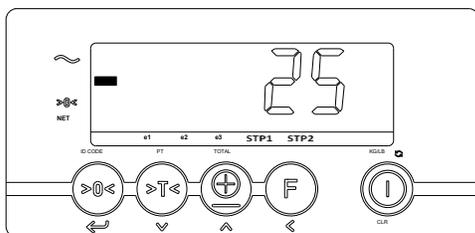
When the pallet wagon is completely unloaded, the tare value is displayed negatively.
