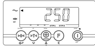
Press the TOTAL key to add the weight load to the total weight.
