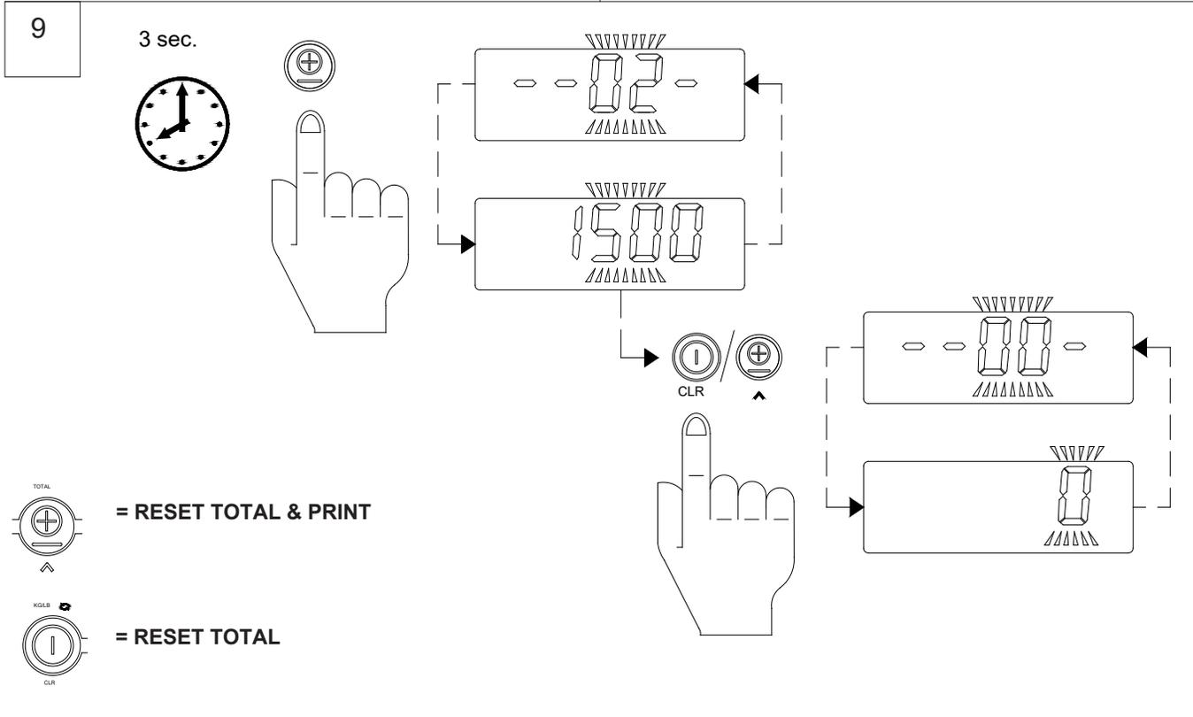
**NOTE:** In case the total is not manually used or reset, the system will do this automatically as soon as the total number has reached 99 or as soon as the total weight has reached a value of 99999 kg.
