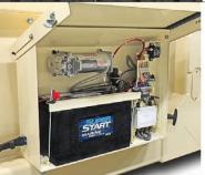
Load cell junction box with additional condensation protection located inside the battery box for easy access.
