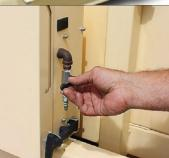
Air purge valve releases air from air bags to easily and quickly lower into weighing mode.
