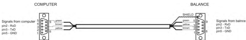
Scale – computer cable (RS232)
