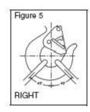
\* For two legged slings with angles greater than 90 degrees, use an intermediate link such as a master link or bolt type shackle to collect the legs of the slings. The intermediate link can be placed over the hook to provide an in-line load on the hook. This approach must also be used when using slings with three or more legs.
