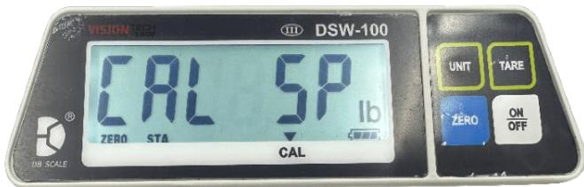
6. Place the calibration weight and press the **ZERO** button.
