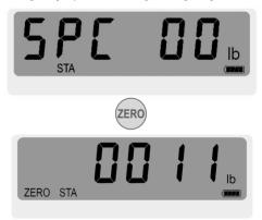
■Click [UNIT] key to modify Spec 00. The display will show SPC 00, and then press the [ZERO] to enter the power saving mode.
